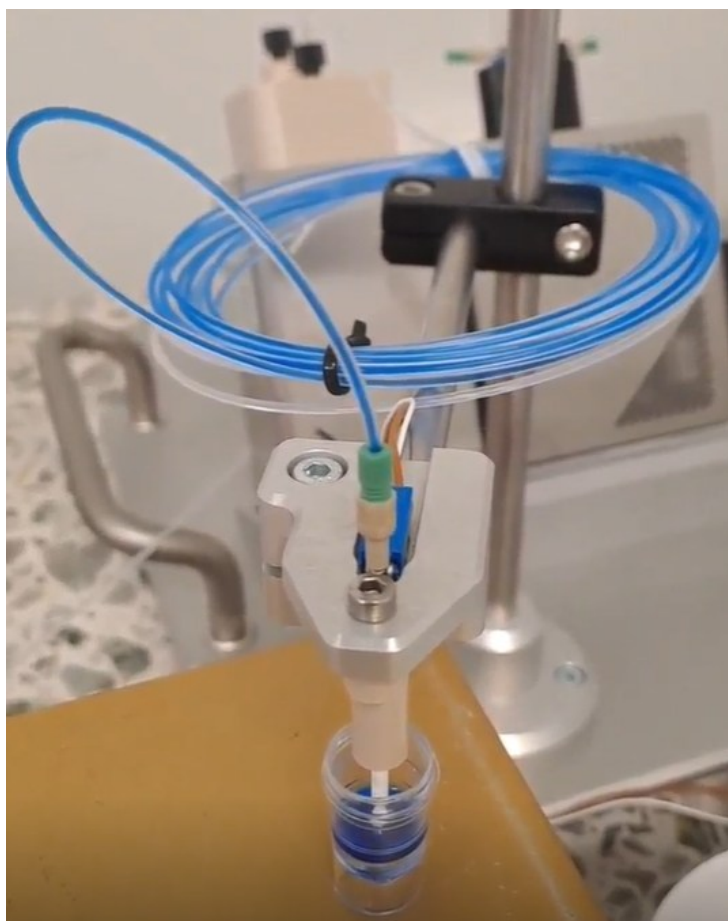
Figure 20 Buffer with dye being aspirated into the dispensing tubing
